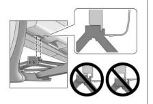
Raise the vehicle by turning the wheel wrench clockwise until the slots in the jack head fit into the metal flange located behind the triangle on the plastic moulding.
